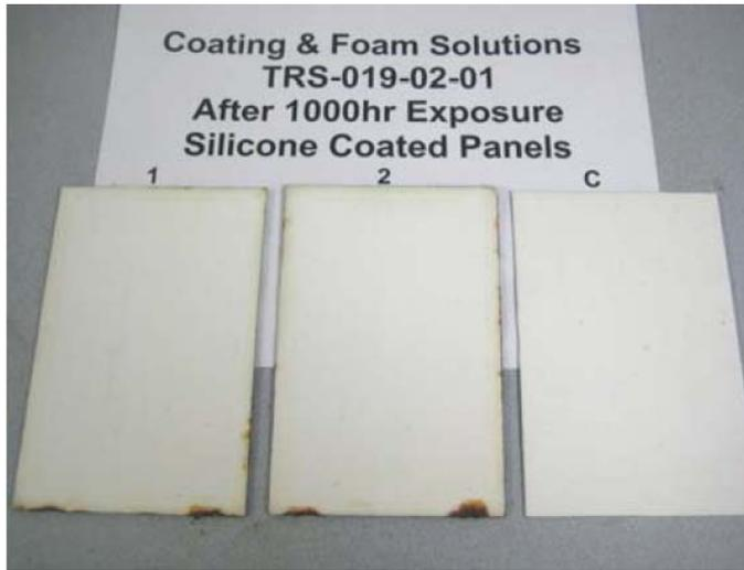
Samples passed ASTM B 117 testing procedure for Corrosion Resistance. Independent lab testing confirmed panels with only 8 mils (dft) of Poly-Sil™ 2200 CC coating successfully achieved over 1000 hours of salt spray exposure.
